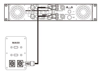
**Note:** The output impedance of speaker and amplifier should be matched.
